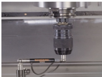
Ball-Bar Testing on every machine
